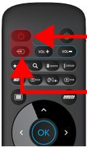
1. On the BT-250, press and hold the TV POWER + TV SOURCE for 3 seconds. Once the blue light turns on, release the buttons.
